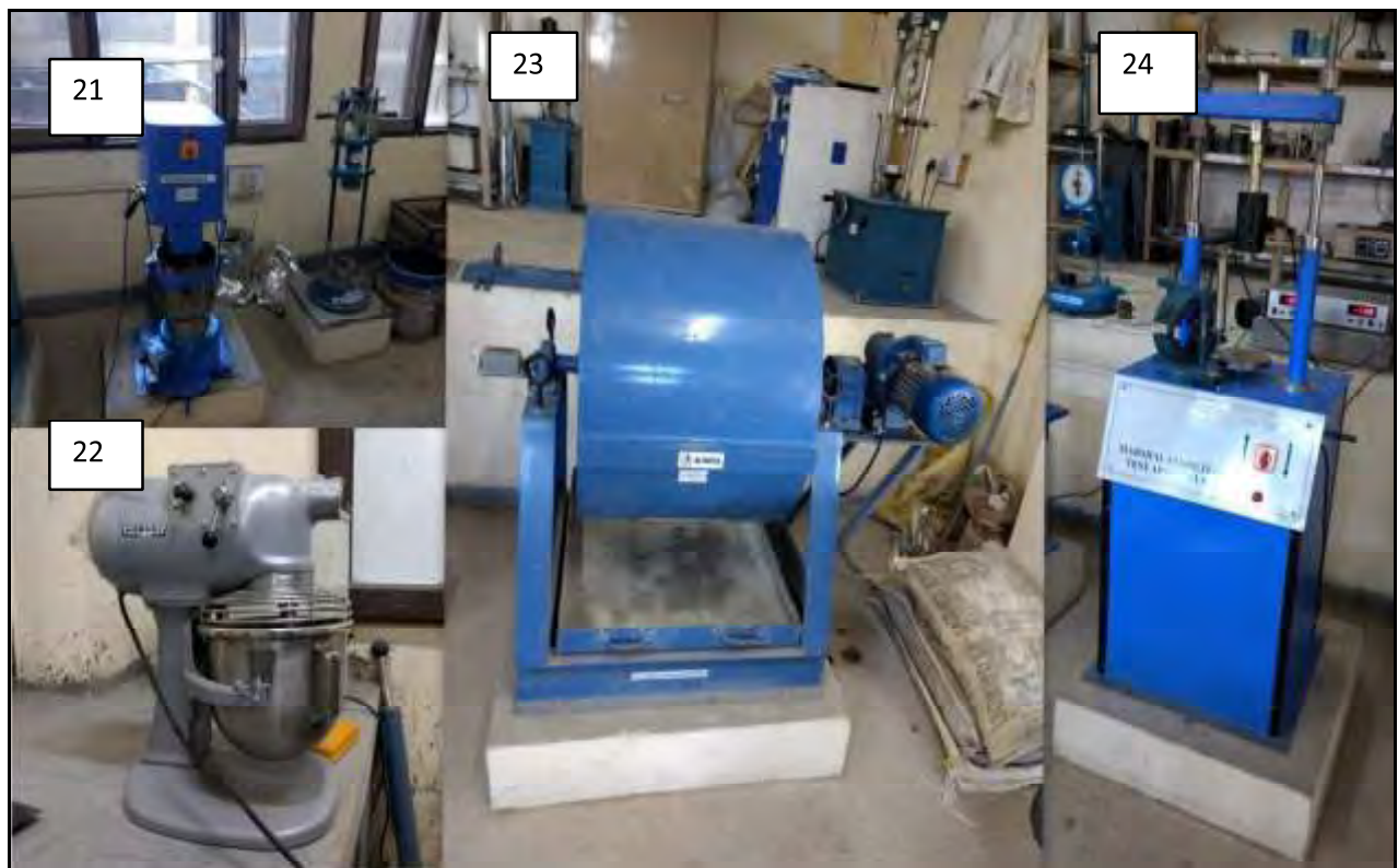
21. Bitumen Mixer/ Impact Testing Machine 22. Hobart Mixer 23. Los angles Abrasion testing machine 24. Marshall Testing Apparatus
