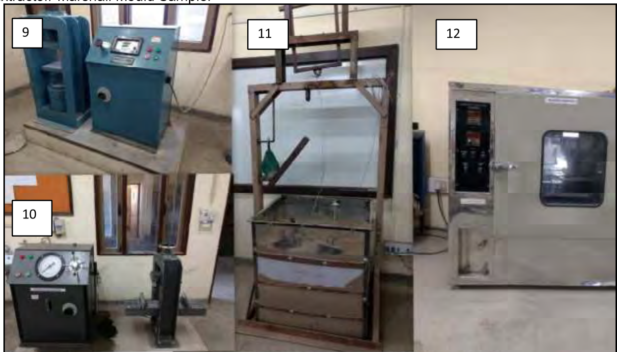
9. Compression Testing Machine 10. Flexural Strength Testing Apparatus 11. Soil Pulling Apparatus 12. Humidity Apparatus
